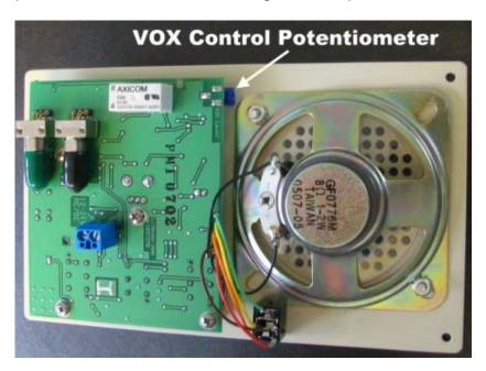
Turning this potentiometer clockwise will increase the sensitivity of this threshold while turning it counterclockwise will decrease the sensitivity.
