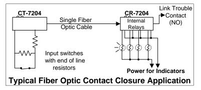
Note that the CR-7204.receiver output contacts are fully isolated from each other and any other terminal.
