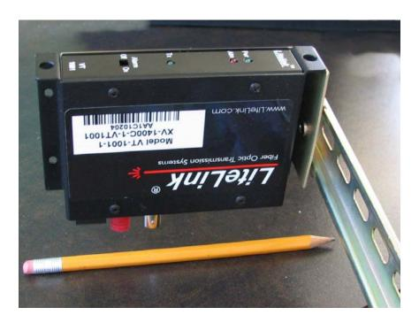
The DIN Rail adapter can be used with any small or medium Liteway product housing to allow mounting of the product to a standard DIN Rail (EN 50 022 or EN 50 035)
